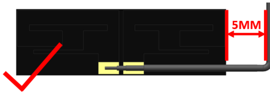
FIGURE 5.2.1 RECOMMENDED CABLE BENDING RANGE
