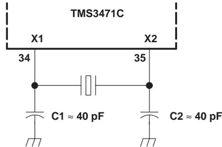
NOTE: The TMS3471C is designed for use with a crystal oscillator. The X1 and X2 terminals should not connect directly to external driver outputs.
