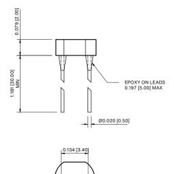
Note: Lead soldering temperature (1/16 inches away from body) 260°C for 3 sec.
