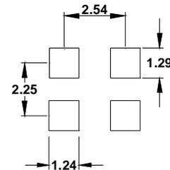
Note: XPRESSO HCMOS XO's are designed to fit on industry standard, 4 pad, layouts.
