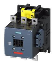
Power contactor, AC-3 265 A, 132 kW / 400 V Coil AC 50/60 Hz and DC 200-277 V x (0.8-1.1) F-SPS input 24 V DC 3-pole size S10 Auxiliary contacts 2 NO + 2 NC permanently mounted Main circuit: Busbar Control and auxiliary circuit: Screw terminal
