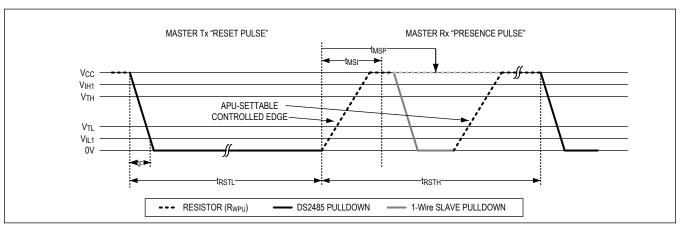
Figure 1. 1-Wire Reset/Presence-Detect Cycle
