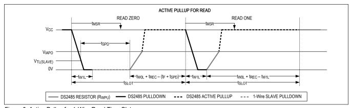
Figure 6. Active Pullup for 1-Wire Read Time Slot
