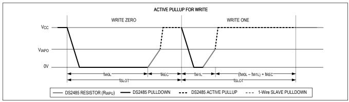
Figure 5. Active Pullup for 1-Wire Write Time Slot
