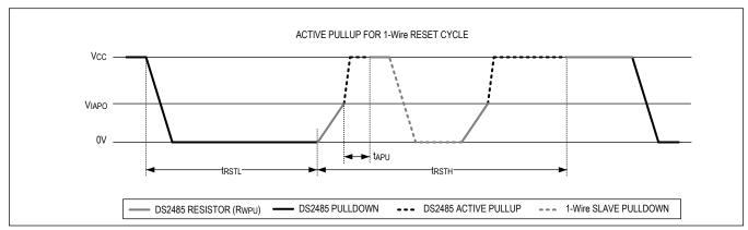
Figure 4. Active Pullup for a 1-Wire Reset Cycle
