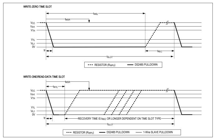
Figure 2. Read/Write Timing Diagrams
