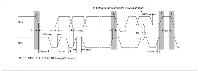
Figure 9. I<sup>2</sup>C Timing Diagram
