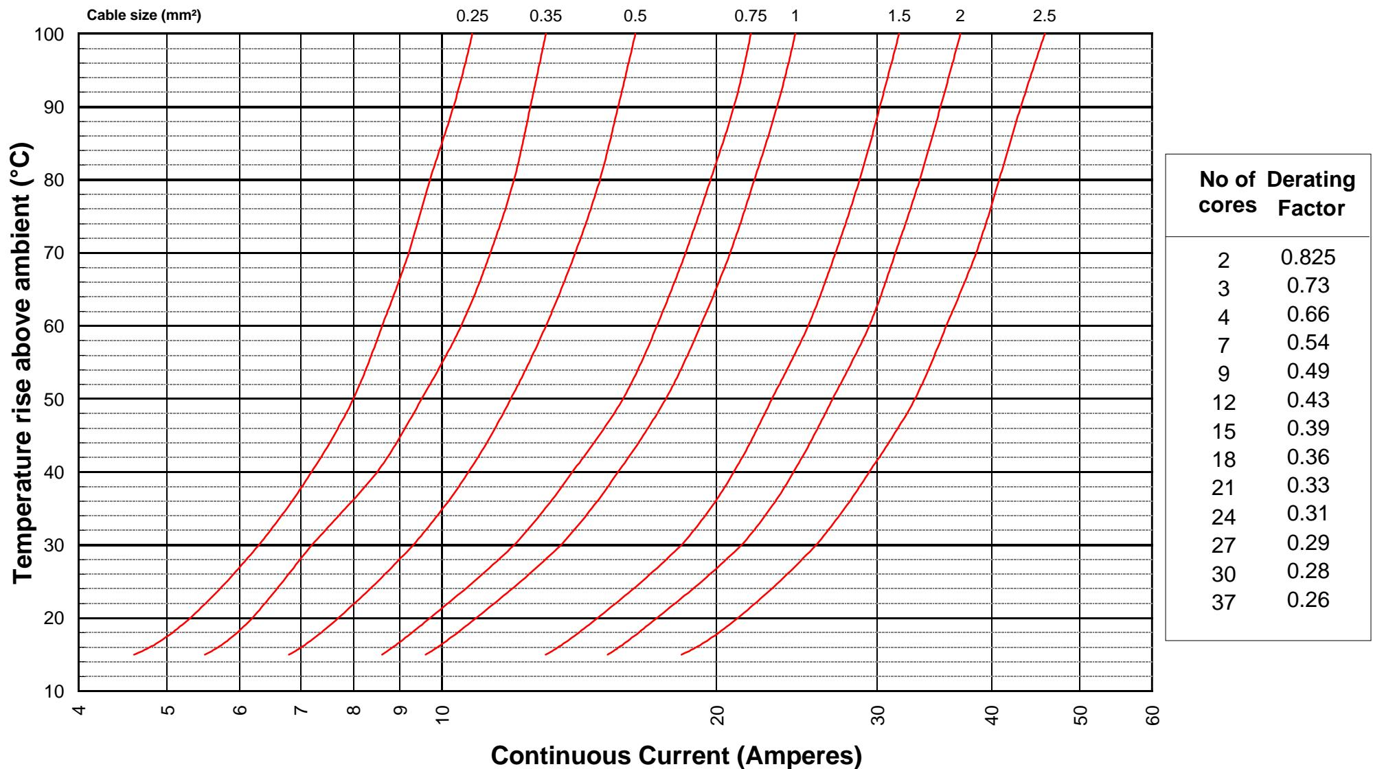
For ambients other than  $20^{\circ}\text{C}$  divide the current by:  $\sqrt{(234.5 + \text{ambient})/254.5}$
