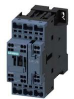
power contactor, AC-3 17 A, 7.5 kW / 400 V 1 NO + 1 NC, 125 V DC with integrated varistor 3-pole, size S0, spring-type terminal suitable for PLC outputs not expandable with auxiliary switch
