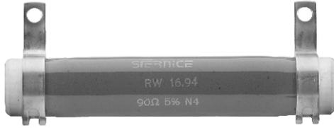
The RW wirewound power resistors are extremely well suited to professional applications, where high power and excellent endurance are required. They meet all requirements of NF C 93-214 specifications and five sizes cover the power range from 10 W to 80 W. Non inductive types are available, by using the special RWN1 winding. For higher power or extremely severe conditions of use, see the RWST series.
