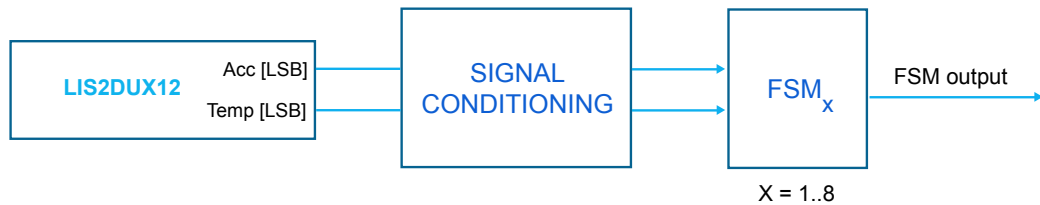
Figure 11. State machine in the LIS2DUX12
