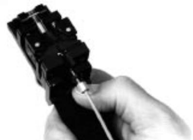
Carefully insert the ferrule into the slot on the diamond cleave tool until the ferrule rests securely in the cleave tool connector adapter.
