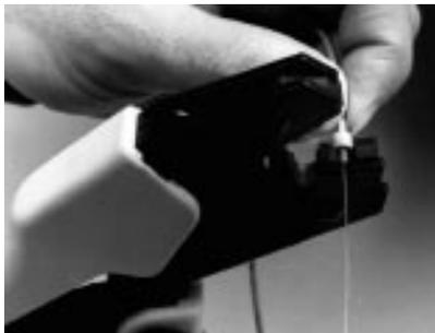
Place the crimp ring over the end of the cable and rest the larger end against the unstripped cable jacket. Selecting the smaller crimp hole (front die nest), align the crimp ring in the crimp tool jaws and fully squeeze the tool handles together and release. This crimps the crimp ring to the fiber buffer.
