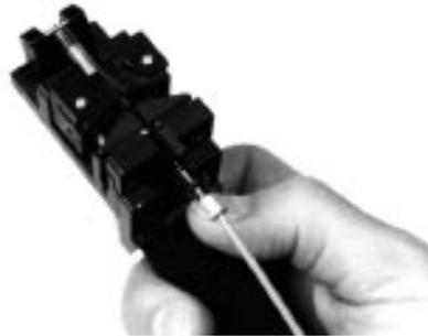
and release the cleave tool trigger. Remove the fiber remnant from the cleave tool fiber clamps and dispose of properly.
