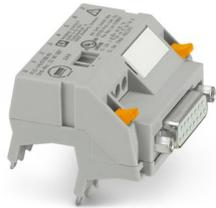
V8 adapter for 8 x PLC-INTERFACE (6.2 mm), controller: PLC system cabling of input cards, connection 1: D-SUB socket strip 1x 15-position, connection 2: Plug-in connection (Can be snapped onto 8x PLC-INTERFACE terminals), connection 3: Screw connection 1x 2-position, number of channels: 8, control logic: positive switching
