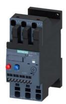
Overload relay 30...36 A Thermal For motor protection Size S0, Class 10 Standalone installation Main circuit: Spring-type terminal Auxiliary circuit: spring-type terminal Manual-Automatic-Reset
