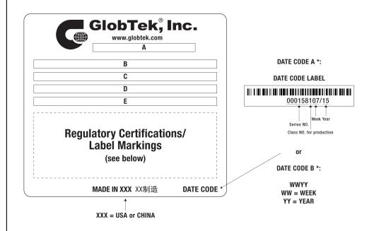
A=ICT / ITE / Medical Power Supply B=P/N: (料号) GTM91110P24024CAS(R) C=Model (型号) GTM91110P24024-CA-S D=Input (输入)100-240V~, 50-60 Hz, 4.0A E=Output (输出)24.0 V == 8.33 A, 200.00W
