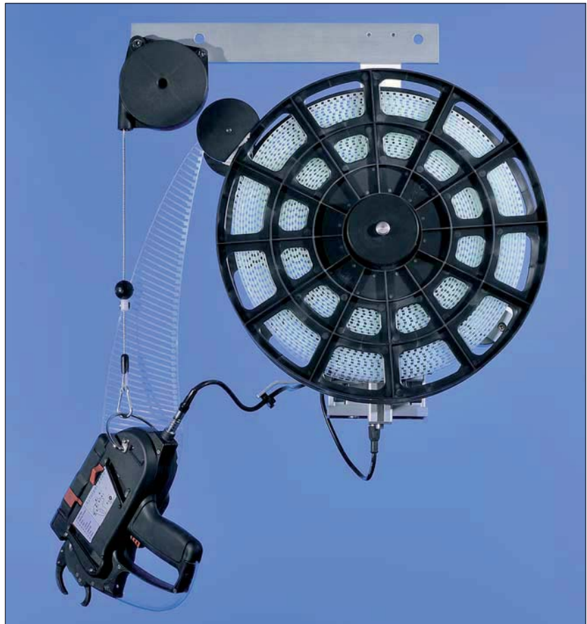
Overhead suspender, reel with ties and Autotool 2000.
