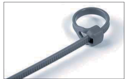
Outside serration means no damage of insulation.
