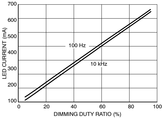
Figure 13. LED Current vs. Dimming Duty Ratio
