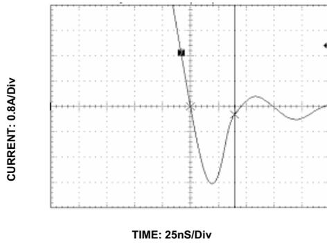
Figure 14. FDMS8670AS SyncFET Body Diode Reverse Recovery Characteristics
