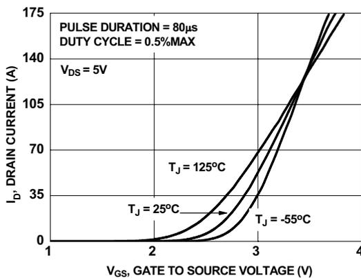
**Figure 5. Transfer Characteristics**
