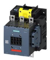
power contactor AC-1 275 A / 690 V / 40  $^{\circ}$ C 3-pole, Uc: 96-127 V AC(50-60 Hz) / DC F-PLC input 24 V DC drive: electronic auxiliary contacts 2 NO + 2 NC main circuit: busbar control and auxiliary circuit: screw terminal
