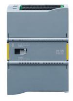
SIPLUS S7-1200 SM 1226 F-DQ 4x24 V DC -25...+55°C with conformal coating based on 6ES7226-6DA32-0XB0 . F-DQ 4x 24 V DC 2A, PROFIsafe, 70 mm overall width, up to PL E (ISO 13849-1)/ SIL3 (IEC 61508)
