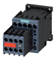
Power contactor, AC-3 16 A, 7.5 kW / 400 V 2 NO + 2 NC, 230 V AC 50/60 Hz, 3-pole Size S00, Screw terminal Auxiliary switch block captive
