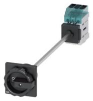
Load disconnector 3LD3, Iu 32 A Main switch 3-pole Rated operating capacity for AC-23 A at 400V 11.5kW floor mounting Basic switch with door coupling Central hole mounting 22.5mm Rotating drive black 66 x 66 mm
