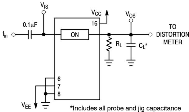
Figure 14a. Total Harmonic Distortion, Test Set-Up
