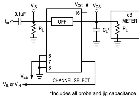
Figure 7. Off Channel Feedthrough Isolation, Test Set-Up
