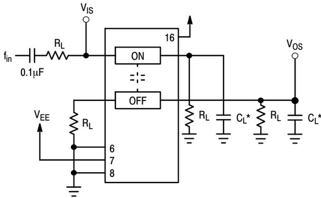
Figure 12. Crosstalk Between Any Two Switches, Test Set-Up
