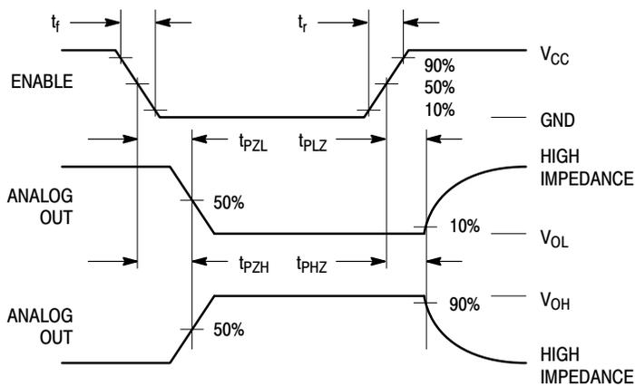
**Figure 11a. Propagation Delays, Enable to Analog Out**
