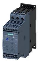
SIRIUS soft starter S0 12.5 A, 7.5 kW/500 V, 40  $^{\circ}\text{C}$  400-600 V AC, 24 V AC/DC Screw terminals
