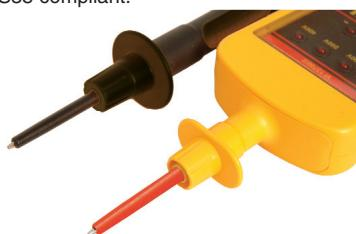
The probe is sealed and the fuse that was in earlier versions has been replaced by a non user serviceable resistor to provide protection if the cable is damaged.
