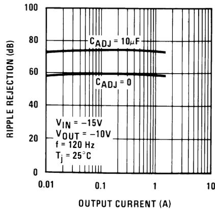
Figure 9. Ripple Rejection
