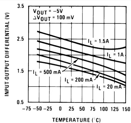
Figure 4. Dropout Voltage
