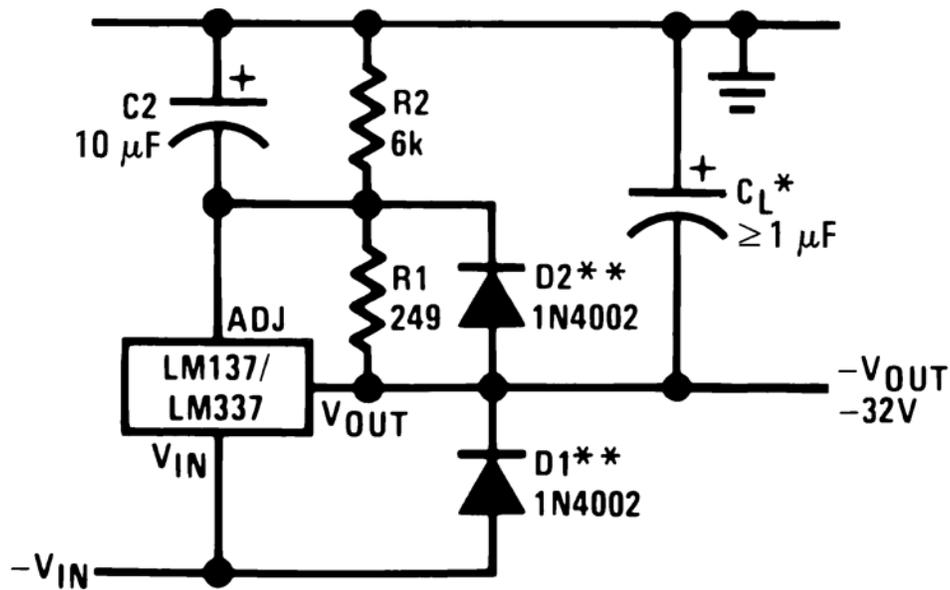
\*When  $C_L$  is larger than 20  $\mu\text{F}$ , D1 protects the LM137 in case the input supply is shorted
