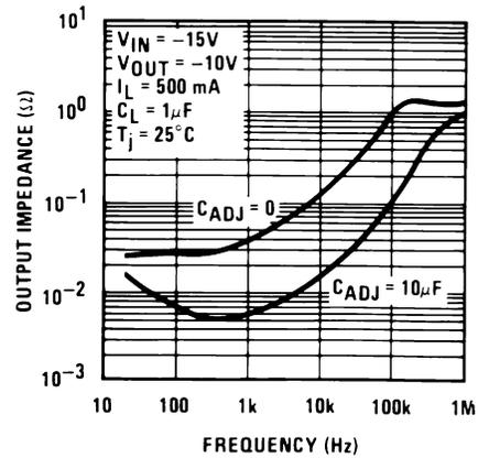
Figure 10. Output Impedance
