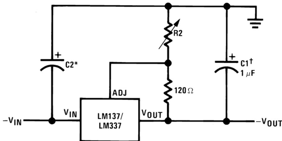
Full output current not available at high input-output voltages
