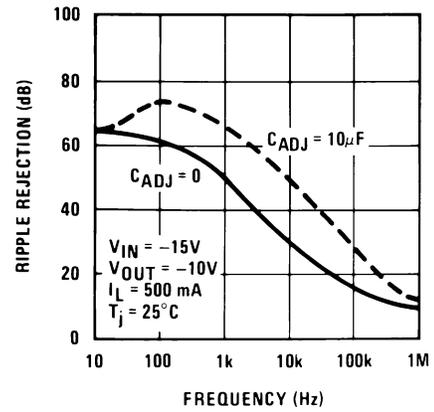
Figure 8. Ripple Rejection
