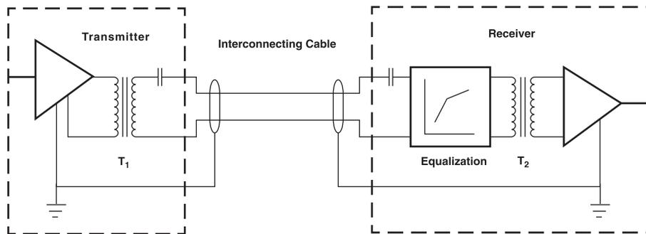
T<sub>1</sub>, T<sub>2</sub>: PE-65612 or PE-65812
