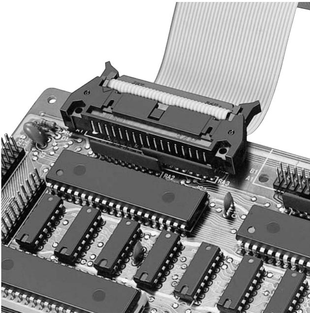
**Contemporary needs require that electronic equipment be high in density, modular in construction and multi-functional. In addition, the costs of such connection systems must be reduced. To meet these needs, particularly in the video and audio fields, we offer JST's highly reliable and cost-efficient RX connectors. These connectors reflect displacement connection technology as well as its advanced production techniques.**
