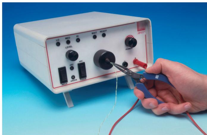
The Thermocouple Welder is a compact, simple-to-use instrument designed for thermocouple and fine wire welding
