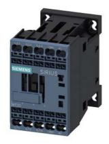
power contactor, AC-3 12 A, 5.5 kW / 400 V 1 NO, 220 V AC, 50 Hz 240 V, 60 Hz, 3-pole Size S00, Spring-type terminal
