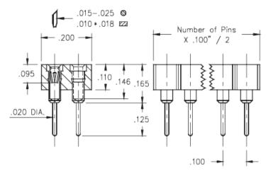
**Description:** Interconnect Socket Standard Solder Tail Socket Accepts .015"- .025" (0,38 - 0,635 mm) dia leads Double Row Through Hole Plating Code:
