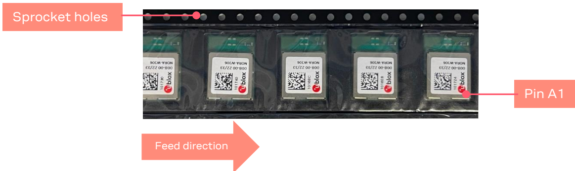
Figure 8: NORA-W366 module on tape orientation
