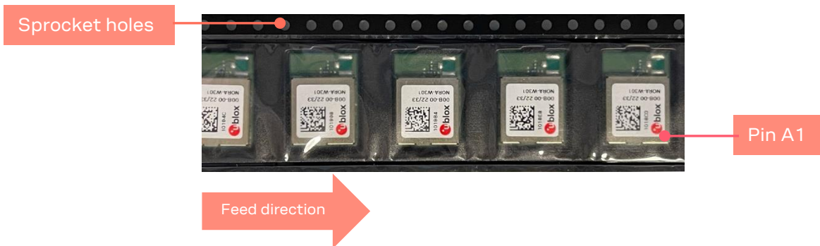
Figure 7: NORA-W361 module on tape orientation
