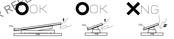
(3) If the FPC is not rigid, The connector can be broken. Please check the action of the FPC to be used repeatedly at the time of trial production, be careful to un-mate them from the pitch direction, pulling it from the corner can also risk to putting stress on contacts.
