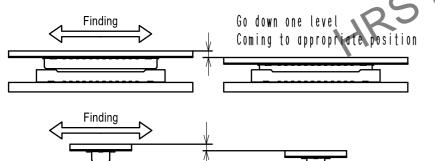
(2) When quiding, the connectors are aligned parallel to each other, with longitudinal and lateral movements restricted. Mate them properly by applying force in this condition.
