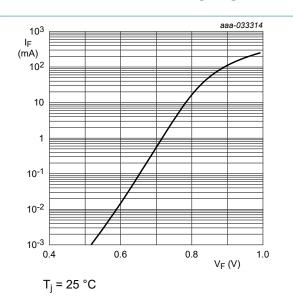
Fig. 2. Forward current as a function of forward voltage; typical values (BZX8450-C1V8)
