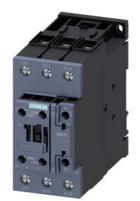
power contactor, AC-3 40 A, 18.5 kW / 400 V 1 NO + 1 NC, 240 V AC 50 Hz, 3-pole, Size S2, screw terminal
