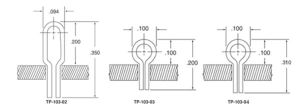
\*Note: Leads flared to provide retention in the printed circuit board.
