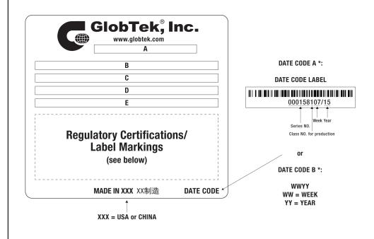
A=ICT / ITE / Medical Power Supply B=P/N: (料号) GTM43007-A6036-F(R) C=Model (型号) GTM43007-A6036-F
