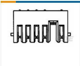
TE Part #1473971-2 REC ASS'Y V TYPE FOR 2.5MM PIT
