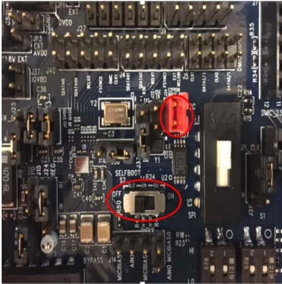
Figure 23. SELFBOOT and Write Protect (WIP) Settings
