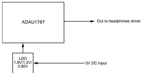
Figure 33. EVAL-ADAU1787Z Schematic: Block Diagram
