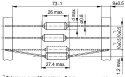
\*) Tolerance over 10 spacings ±2 mm IND0150-S-E
