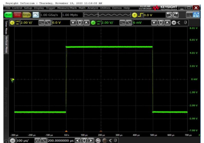
Figure 16. Negative Overload Recovery
