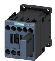
power contactor, AC-3 12 A, 5.5 kW / 400 V 1 NO, 24 V DC 0.85-1.85\*US with varistor plugged on 3-pole, size S00 screw terminal not expandable with auxiliary switch
