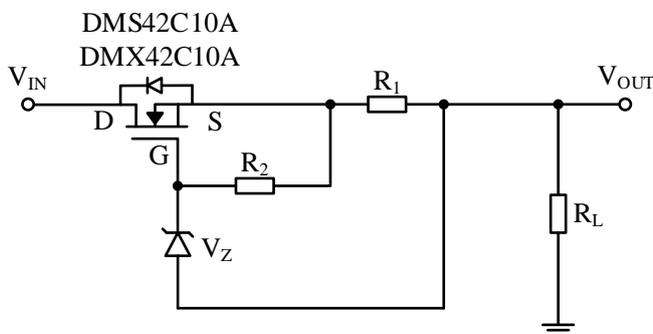
**Figure 11a. Constant current source/ Overcurrent protection**
