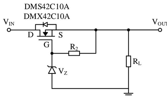
**Figure 12: Voltage regulator/Overvoltage protection**
