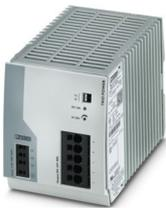
Primary-switched TRIO power supply for DIN rail mounting, input: 3-phase, output: 24 V DC/40 A, dynamic boost, tool-free fast connection technology for solid and stranded conductors with ferrule
