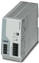
Primary-switched TRIO POWER power supply with push-in connection for DIN rail mounting, input: 3-phase, output: 24 V DC/20 A
