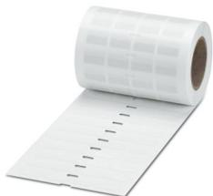
Equipment marking, Roll, white, unlabeled, can be labeled with: THERMOMARK E.300 (D)/600 (D), THERMOMARK ROLL 2.0, THERMOMARK ROLL, THERMOMARK ROLL X1, THERMOMARK ROLLMASTER 300/600, THERMOMARK X1.2, mounting type: adhesive, lettering field size: 20 x 7 mm, Number of individual labels: 4000
