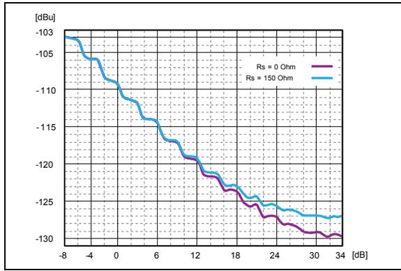
Figure 3. 6261 EIN vs. gain, 0Ω and 150Ω termination.
