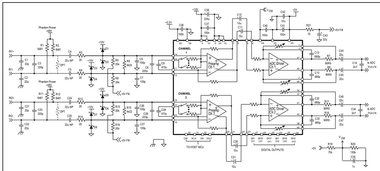
Figure 20. A typical unipolar-supply THAT626x application circuit.
