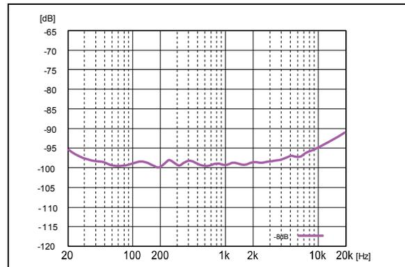
Figure 8. 6261 ADC driver stage VAD PSRR vs. frequency.
