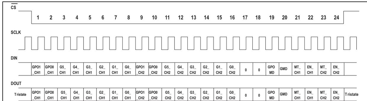
Figure 14. 626x 24-bit SPI control word definition.
