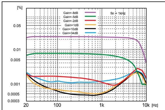
Figure 7. 6261 THD+N at Vout=1.8Vrms vs. frequency, 22kHz BW.
