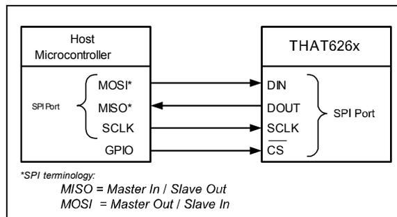
Figure 13. Single 626x connected to a host controller.
