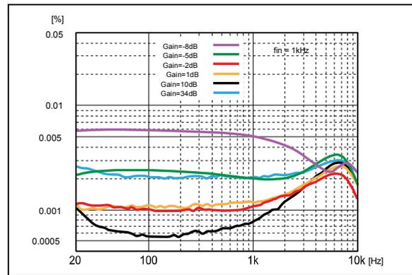
Figure 6. 6261 THD+N at Vout=1Vrms vs. frequency, 22kHz BW.
