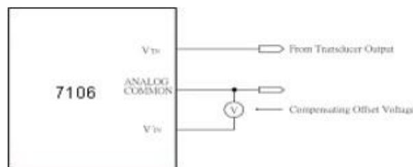
An external reference may be added to improve temperature stability; thus, the HT7106A device with lower analog common temperature drift may be used. See the circuits below:
