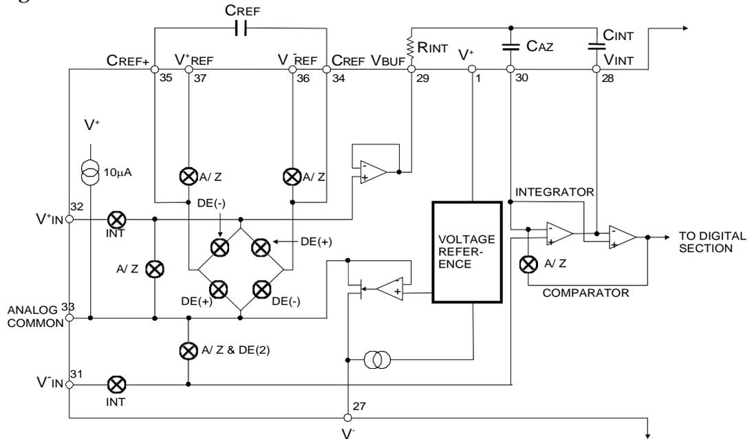
Above is the block diagram of the Analog Section for HT7106A.
