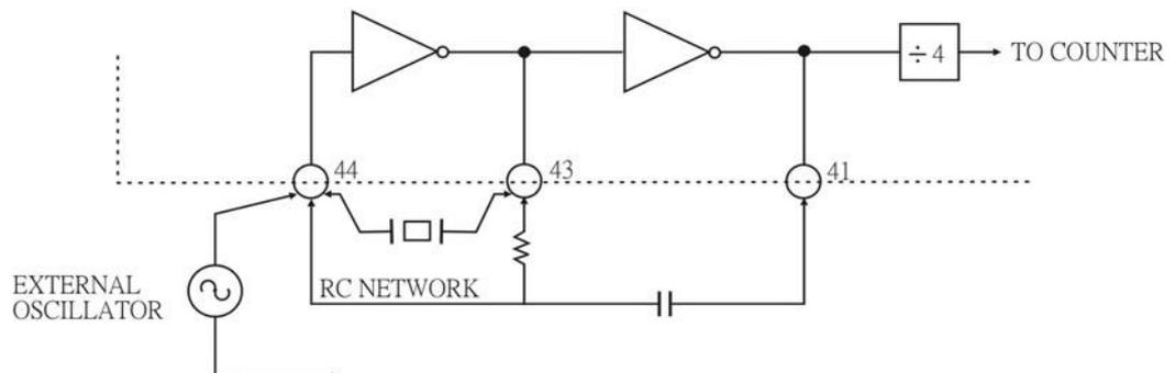
To achieve maximum rejection of 50/60 Hz pick up, the signal integrate cycle should be a multiple of 50/60 Hz. The following table describes the selection of oscillator frequencies for 50 or 60 Hz respectively.
