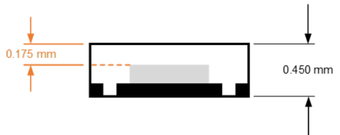
Figure 15: XtremeSense TMR Sensor Location in z Dimension for CT100 in DFN-6 Package
