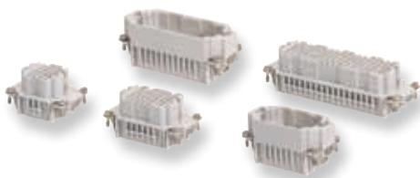
High contact density in the most compact space – this is what the space-saving contact inserts of *revos* DD offer. The inserts fit into the BASIC housing sizes 6/6H, 10/10H, 16/16H, 24/24H. Connection is made with the proven turned crimp contacts, with a diameter of Ø 1.6 mm, which offer a connection range from 0.14 to 2.5 mm<sup>2</sup> at a rated voltage of 250 V (600 V CSA/UL).
