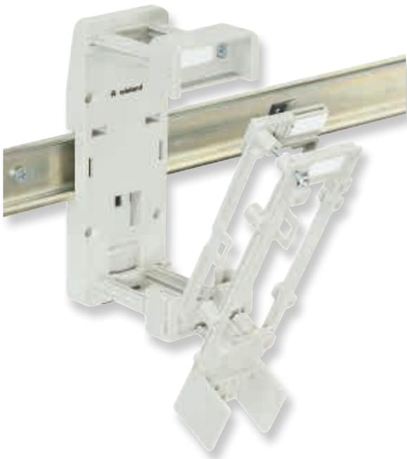
The mounting frames of the **revos** BASIC family are ideal for use in low-voltage switching systems. They are mounted directly to the 35x15 DIN rail according to DIN EN 50022 inside the control cabinet. Use of the DIN rail mounting frame on a 7.5 mm high DIN-rail 35 x 7.5 in accordance with DIN EN 50022 is only possible if the installation space behind it is free.
