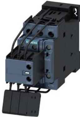
Capacitor contactor, AC-6b 25 kVAr, / 400 V 1 NO + 2 NC, 50-60 Hz AC
