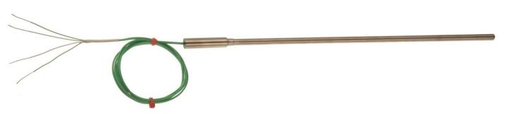
Duplex Type 'K' Thermocouple with two independent measuring junctions inside tip of probe. This allows one probe to be connected to two measurement or control devices; alternatively, one sensor may be used as a primary and the other as a backup, eliminating the need to remove and replace the probe if one of the sensors should fail.
