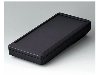
A9075119 DATEC-MOBIL-BOX L, Vers. I ABS (UL 94 HB) black RAL 9005 9.92"x4.76"x1.97" IP 65 opt.
